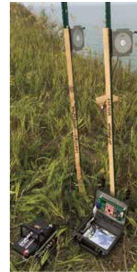
A bluff assessment data generating experiment recorder, also known as a BADGER, ready for work. A BADGER can measure how fast a bluff is moving, soil humidity and temperature, and air humidity and temperature.
